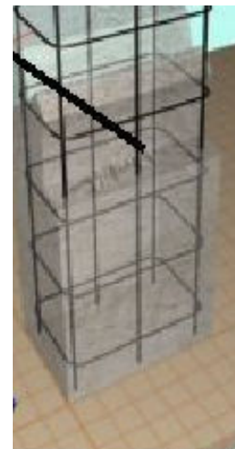
Examples of 3D imaging of rebars after data post-treatment
